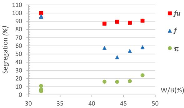
**Figure 3.** Evolution of the segregation index ( $f_u, f$  and  $\pi$ ) with W/B ratio
