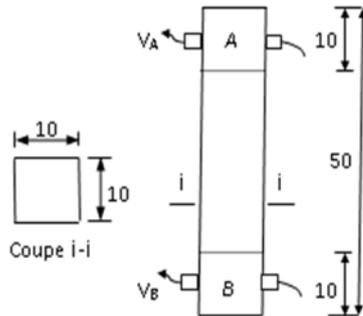
**Figure1.** Velocity propagation on side [A] and [B]: Direct transmission mode.
