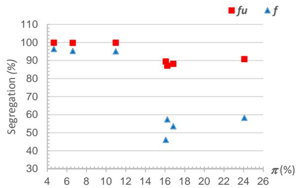
**Figure 5.** Evolution of the segregation index ( $f_u$  and  $f$ ) with  $\pi$  (sieve)
