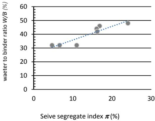
**Figure 2.** Relationship between the sieve segregation index test and the ratio of water-to-binder W/B (based on Table.6)
