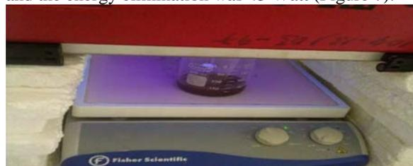
**Figure 7**: Test of photodegradation (Vat Green 3 textile) of titanium dioxide + P25 Degussa (DMF1) in the photocatalytic reactor (transilluminator).
