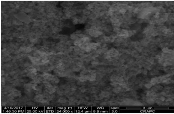
Figure3. Scanning electron microscopy images of TiO<sub>2</sub> nanoparticles deposited on glass plates.
