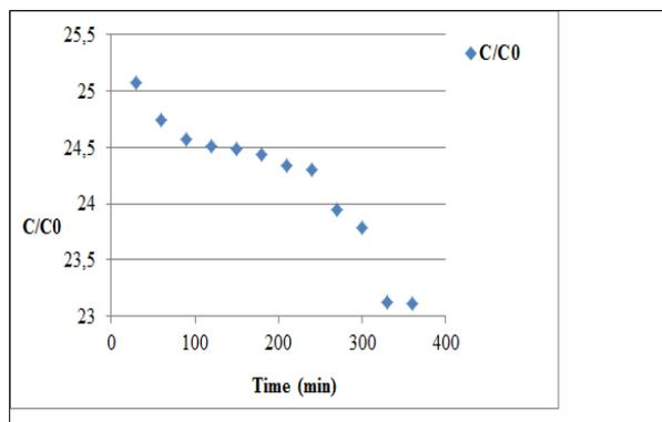
Figure5. Kinetics of degradation of Red Congo by photocatalysis (TiO<sub>2</sub> / UV).
