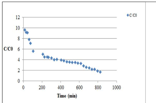
Figure 4. Kinetics of degradation of Malachite green by photocatalysis (TiO<sub>2</sub> / UV).
