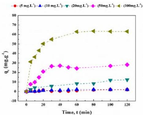
Figure 2. Effect of contact time and initial DS concentration on the removal of DS
