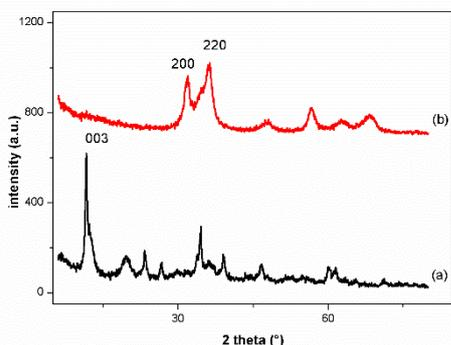
Figure 1. XRD pattern of (a) not calcined LDH (b) calcined LDH.
