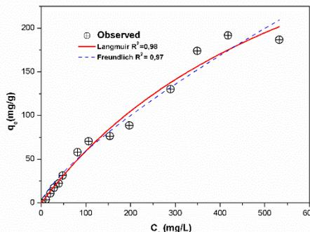
Figure 3. Adsorption isotherm of DS onto calcined LDH.
