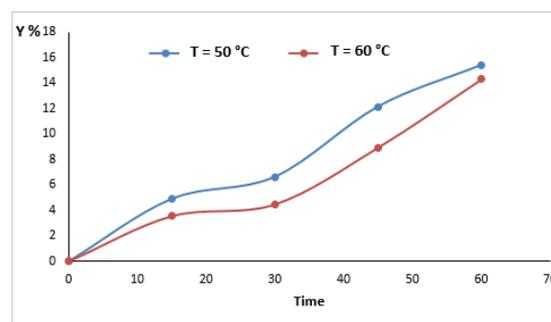
Figure 4: Temperature effect on oil yield at P=300 bar.
