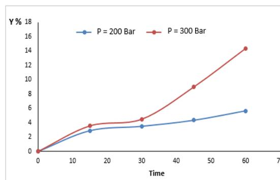
Figure 2: Pressure effect on yield at T=60 °C.
