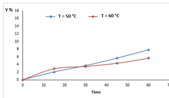
Figure 3: Temperature effect on oil yield at P= 200 bar.
