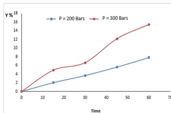
Figure 1: Pressure effect on oil yield at T=50 °C.
