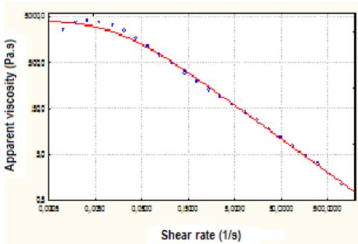
Figure 1. Flow curve of GTW-Hydrogel, T = 20 ° C.
