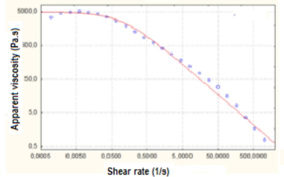
Figure 2. Flow curve of GTW-Hydrogel stored at 4°C for 8 months, T = 20 ° C.
