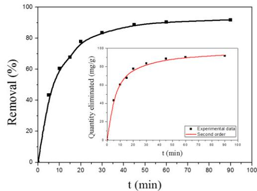
Figure 4. Kinetic of Cr(VI) removal by Amberlite IRN150 resin (C<sub>Cr(VI)</sub>: 100mg/L; resin dose: 1g/L; pH: 5)
