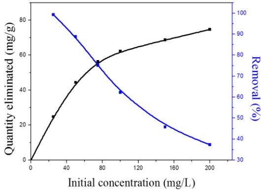
**Figure 5.** Effect of initial concentration on Cr(VI) removal of by Amberlite IRN150 resin (t: 60min; resin dose: 1g/L; pH: 7)
