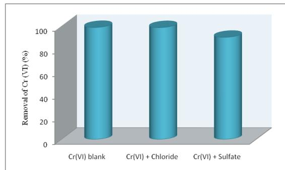
**Figure 7.** Cr(VI) removal by Amberlite IRN150 in the presence of competitor ions (C<sub>Cr(VI)</sub>: 50mg/L; t: 60min; resin dose: 1g/L; pH: 5)
