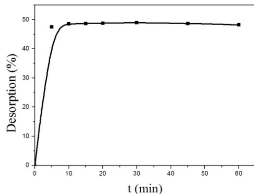
**Figure 8.** Kinetic of Cr(VI) recovery from Amberlite IRN150 by KCl
