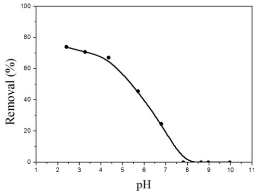
Figure 2. Effect of pH on Cr(VI) removal by Amberlite IRN150 resin (C<sub>Cr(VI)</sub>: 200mg/L; t: 60min; resin dose: 1g/L)
