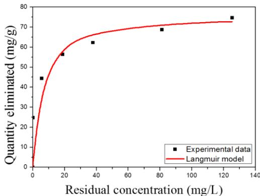
**Figure 6.** Isotherm of Cr(VI) removal by Amberlite IRN150 resin (t: 60min; resin dose: 1g/L; pH: 7)
