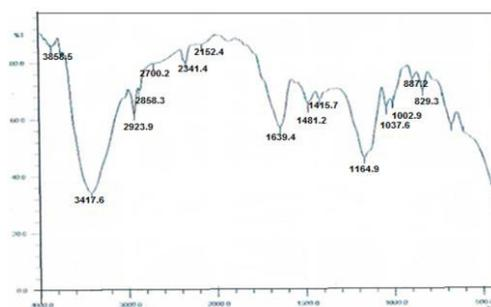
Figure 1. FTIR spectrum of Amberlite IRN150
