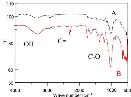
Figure 1. FTIR spectrum of the *L. Cylindrica* fibers (a) without adsorbed Zn(II), (b) with adsorbed Zn(II).
