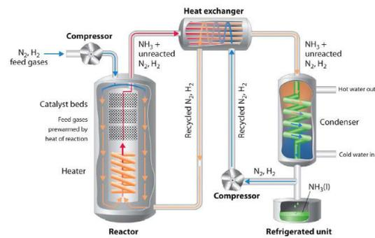
Figure 1. Schematic diagram of an ammonia reactor.
