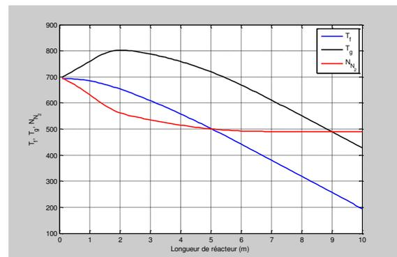
Figure. 3. Profiles of  $N_{N_2}$ ,  $T_f$  and  $T_g$  vs Reactor Length
