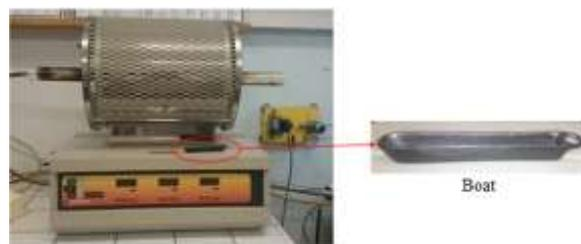
Figure 1. The tubular furnace
